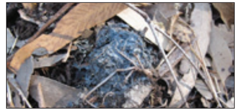
Blue asbestos (friable)
